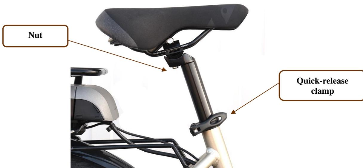
Wearing suitable cycling shoes, sit on the saddle, place one of the pedals in the lowest position, rest one heel on the pedal, and your leg should rest normally on the pedal without being stretched. Raise or lower the saddle to get the correct height. While pedalling backwards, you should not have to move your hips from side to side.
