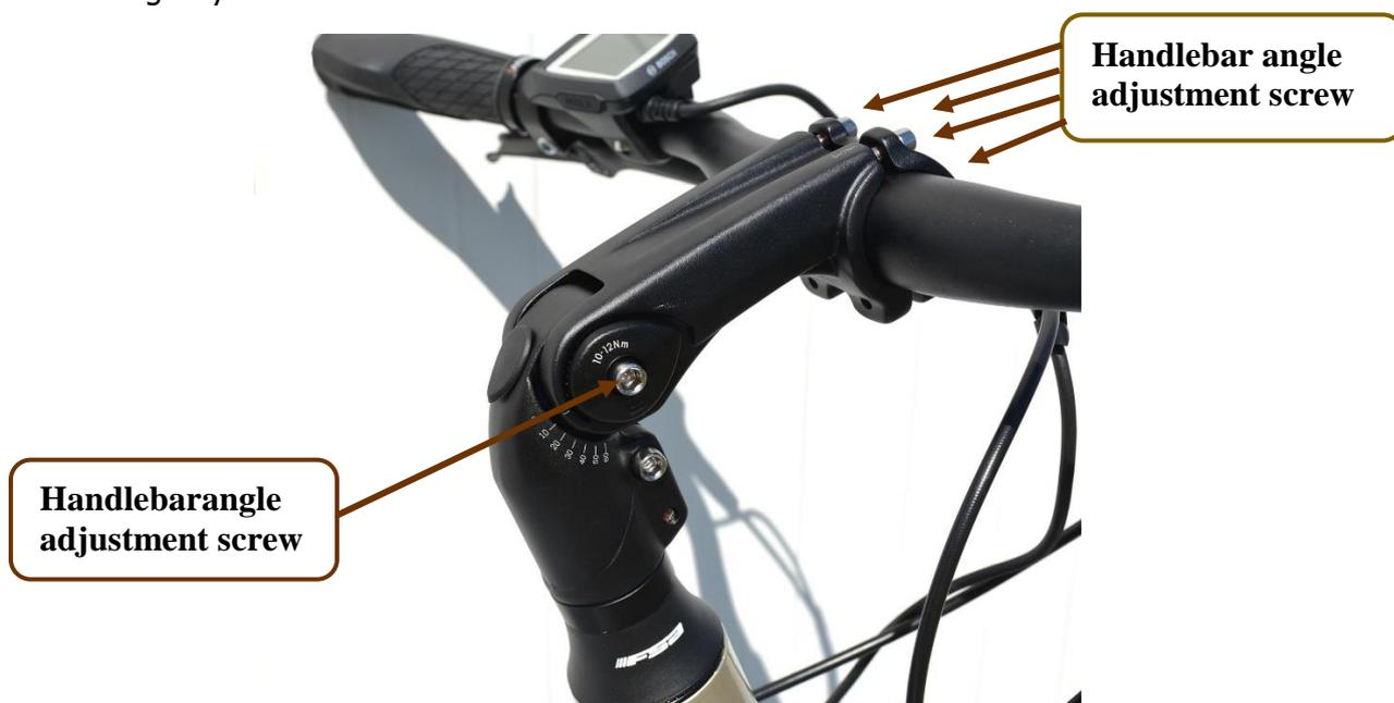
Do the same with the second screw to set the angle of your handlebars, after making your adjustments, tighten the screws vigorously, with a max. tightening torque of 10 Nm.
