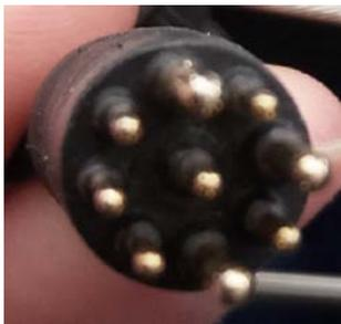
**Position the two pins correctly to reconnect the motor plug**
